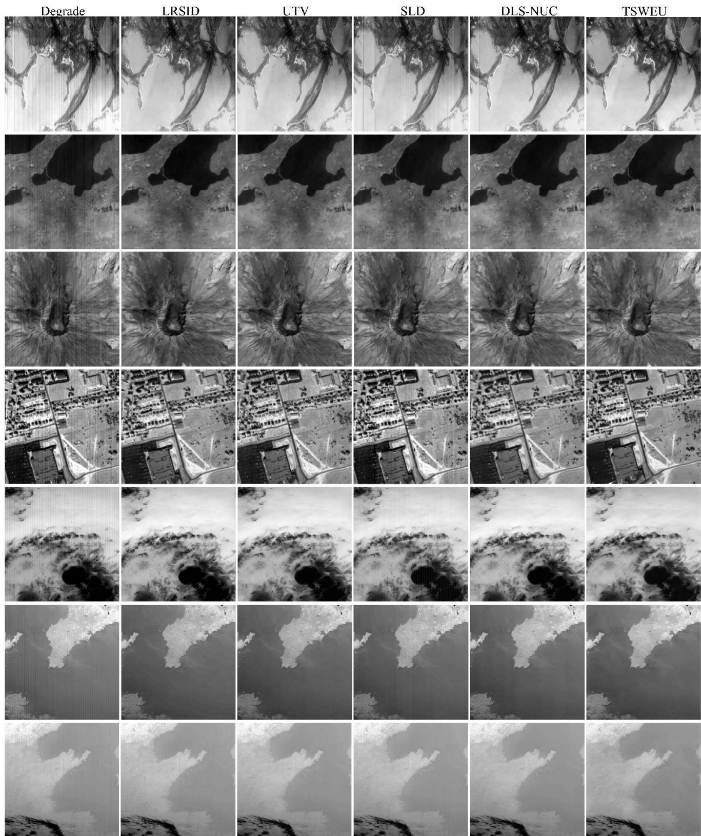
Fig. 15. Real destriping results for various remote sensing images. (From left to right) Real degrade image, the destriping results of LRSID, UTV, SLD, DLS-NUC, TSWEU. (From top to bottom) Hyperspectral image CHRIS band41, LakeMonona band105, MtStHelens band117, Urban band103, and the MODIS image Terra band27, Terra band30, Terra band33.
